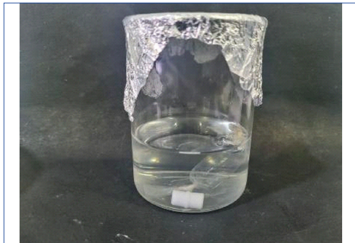
[Table/Fig-4]: A2M Hydrogel inside dialysis membrane submerged in PBS for drug release analysis.
